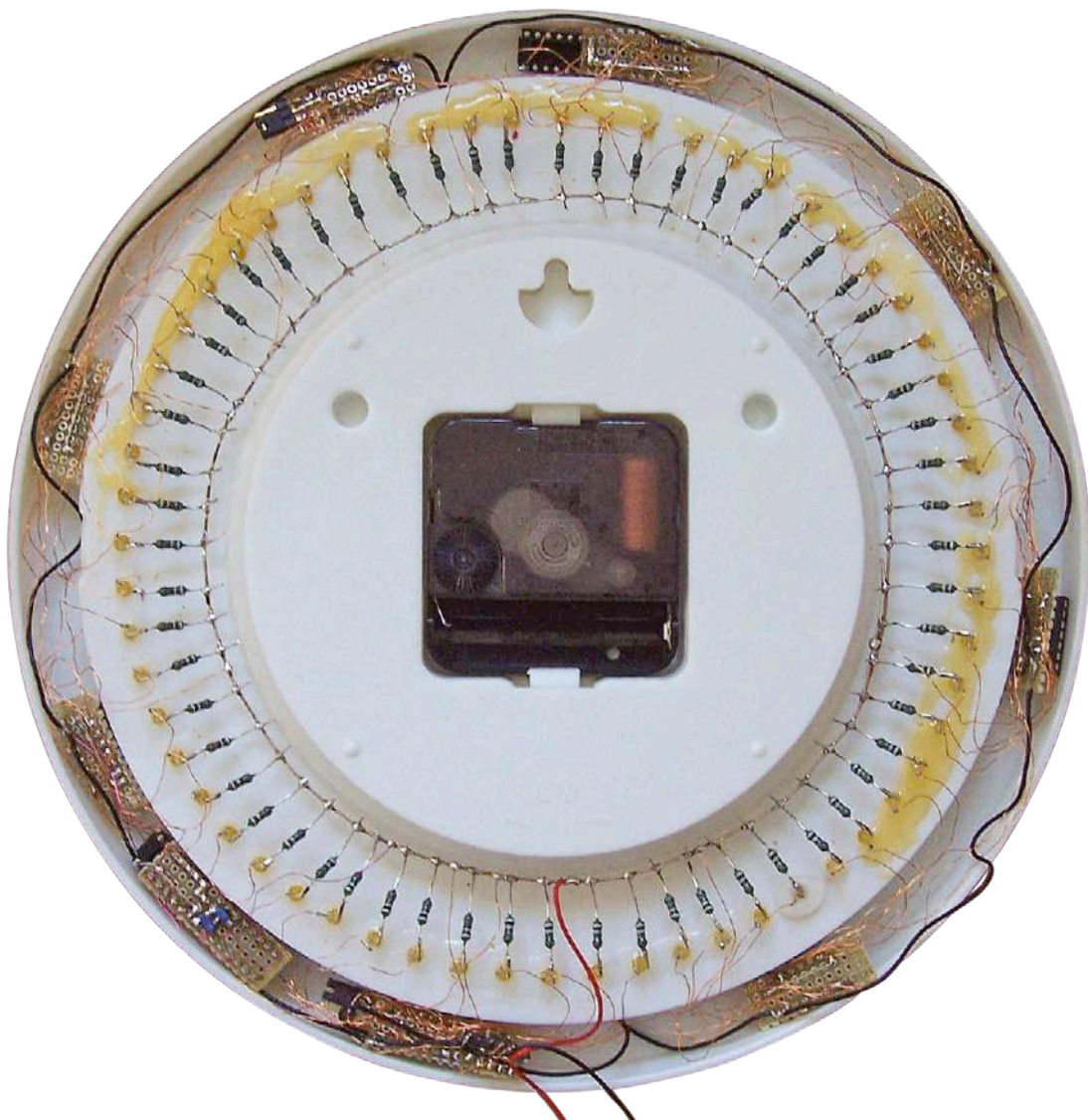
Figure. 4. Wiring the 60 LEDs to the shift registers.
